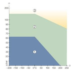
In area 10 the gasket material is suitable using common installation practices subject to chemical compatibility.
